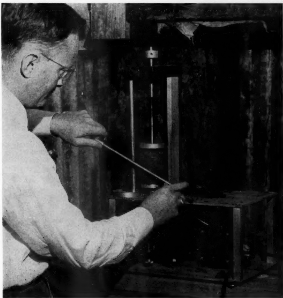
Sawing one of the cylindrical samples down to size, Bonar uses the soil lathe, his newest piece of equipment. Excess dirt is trimmed off with a small wire saw as the whirring lathe spins the sample.
